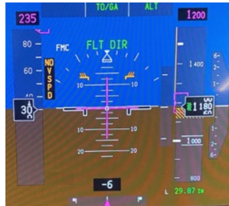
Flight Director ON and MCP Selected Altitude with 20 feet of indicated altitude
