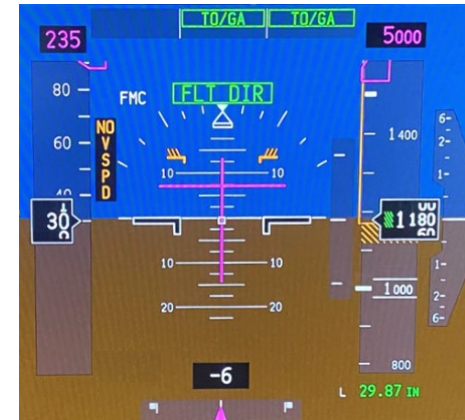
Roll and pitch FMAs show TO/GA, TO/GA when FD switch is selected ON
