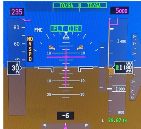
Proper TO/GA guidance will be restored by cycling both F/D switches OFF then ON
